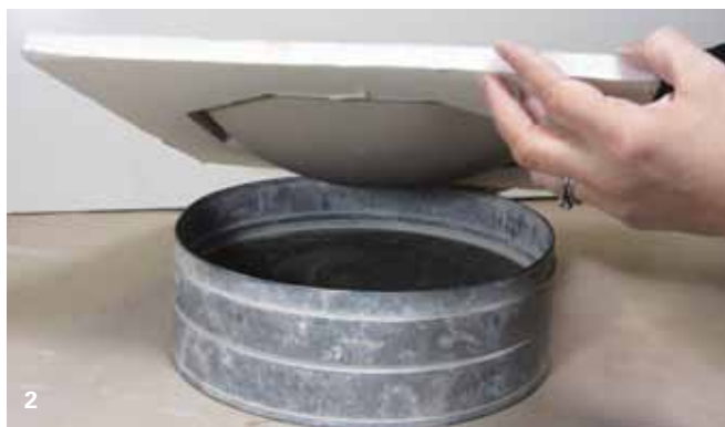
2 Cut away excess clay, leaving only an inch of overlap. Tap the clay, mold, and support on the table causing the clay to slump.
