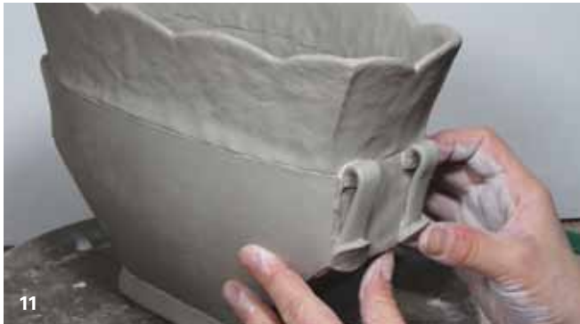
11 Create and attach four small handles and four small petal forms. Attach two to each side by scoring and slipping.
