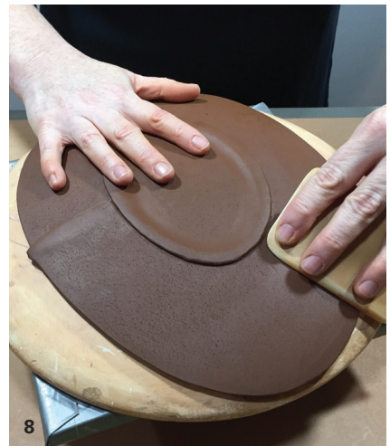
8 Compress the plate face onto the mold to help eliminate warping during the firing.
