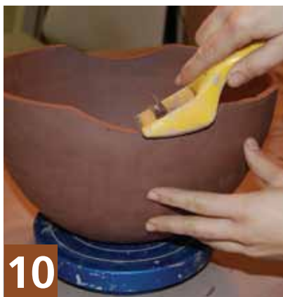
Remove clay down to marks and create a gradual curve to the rim.
