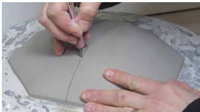
4 Trim the clay to the line left by the board. Draw and cut a line across the middle of the piece.
